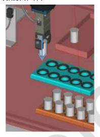
2) Move down into Assembly Tray to insert Cylinder into Ring
