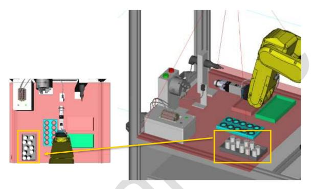
The original Part input tray has fixed locations for the parts.原来的零件输入托盘有零件的固定位置。 This was common practice in industry but is an expensive way to present the parts. 这在工业上是很常见的做法,但这是一种昂贵的展示部件的方式。
